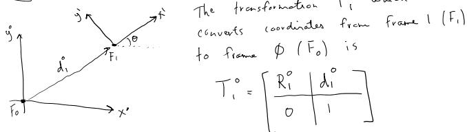
$$T_1^0 = \begin{bmatrix} R_1^0 & d_1^0 \\ 0 & 1 \end{bmatrix}$$
